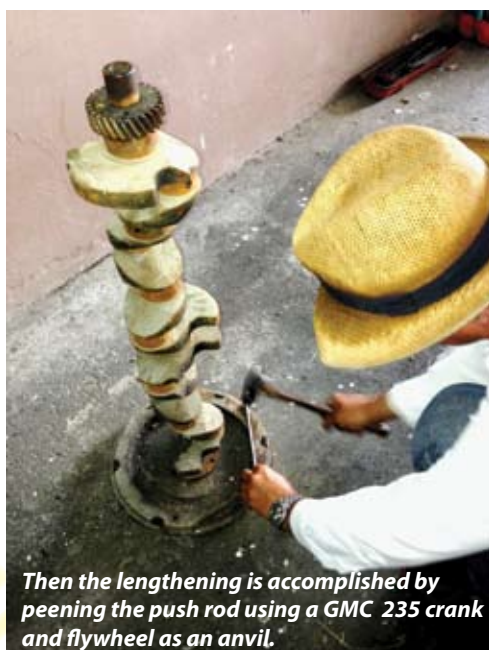
Did you ever adjust your valves by lengthening the push rods? The process starts with careful measurement.
