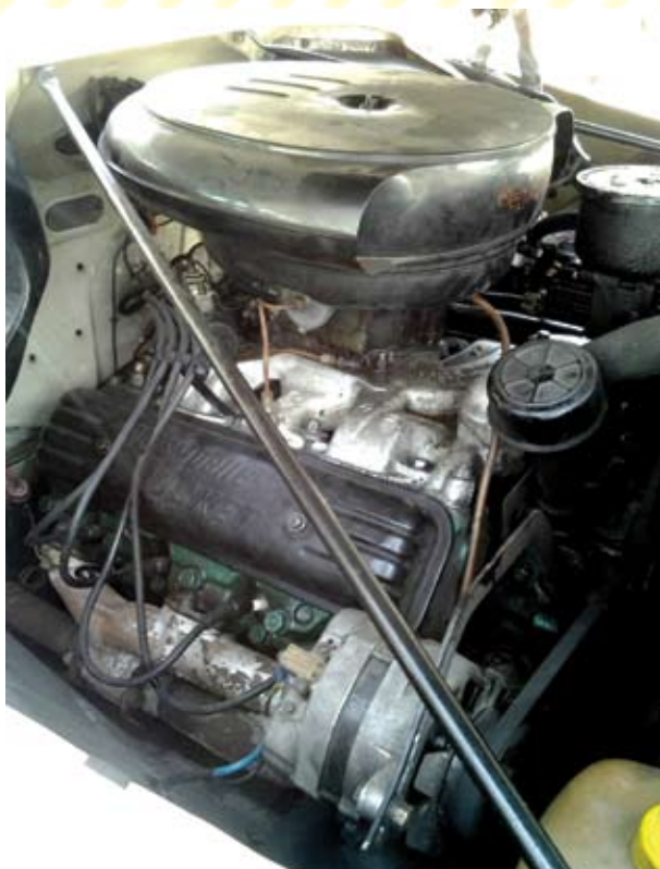
A rare sight in a Cuban Olds: a stock engine with Mercedes valves, Chevy lifters, Cadillac pushrods and Land Rover timing gear and chain
