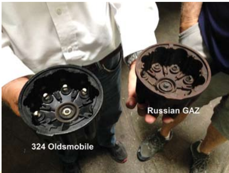
Distributor comparison: 324 Oldsmobile with Russian GAZ
